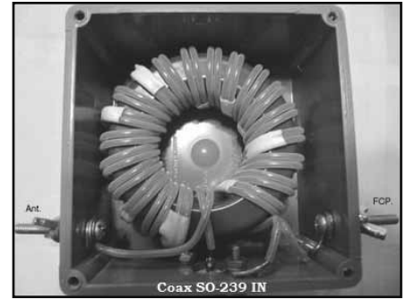
Figure 4 — The K8OZ isolation transformer
